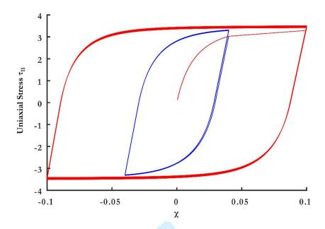
Fig. 7: Tension-compression: Two- sided cyclic loading; non-linear kinematic hardening
