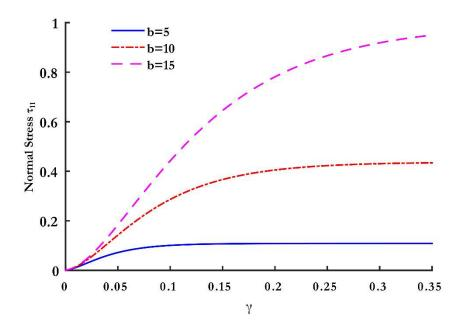
696 Fig. 2: Simple shear: Normal stress  $\tau_{11}$  vs. shear strain  $(\gamma)$ .
