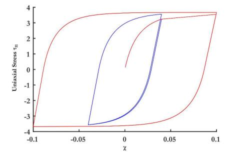
710 Fig. 8: Tension-compression: Two- sided cyclic loading; perfect plasticity.
