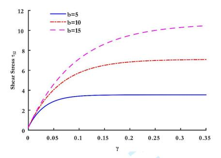
694 Fig. 1: Simple shear: Shear stress  $\tau_{12}$  vs. shear strain  $(\gamma)$ .
