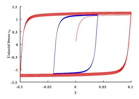
704 Fig. 6: Tension-compression: Two- sided cyclic loading; non-linear kinematic hardening 705 ( $\beta$ =1).
