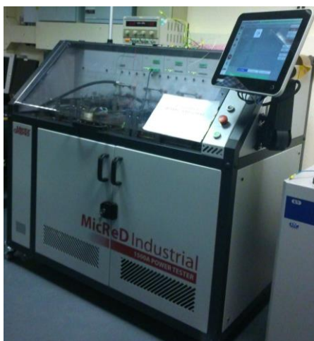
Fig. 1 Power cycling test equipment “Mentor Graphics Power Tester 1500A”
