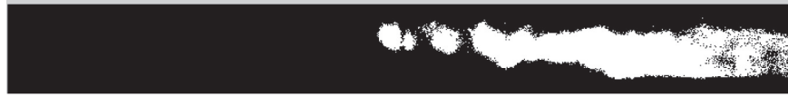
Fig. 5. Result of converting the grayscale image in Fig. 4b to a binary image using im2bw function with a threshold level of 0.12. The image is from the combustion of 75–106 \mu\text{m} pine particles.
