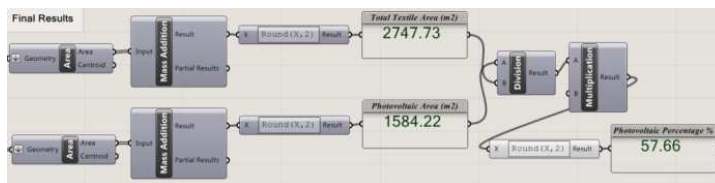
Fig.12: Calculating clear membrane area for PV integration (Ayman Wagdy©)
