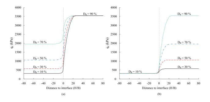
FIG. 6. Cone tip resistance in two-layered ( $D_R$ ) soils: (a) variation of weaker soil; (b) variation of stronger soil
