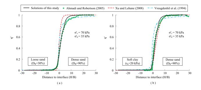
FIG. 9. Comparison of cone tip resistance ratio ( $\eta'$ ) in two-layered soils: (a) loose sand over dense sand; (b) soft clay over dense sand
