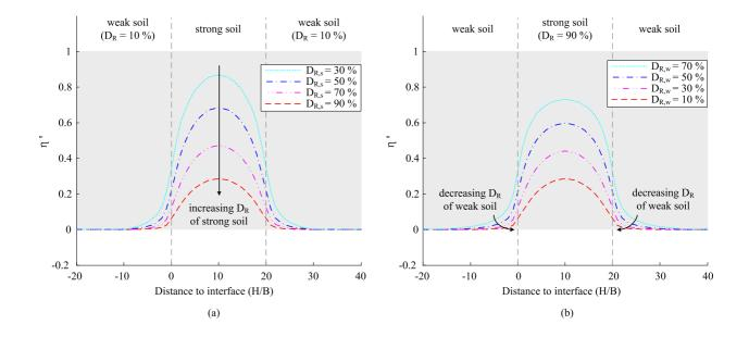
FIG. 13. Resistance ratio curves for thin-layer of strong soil ( $H_t/B = 20$ ): (a) varying  $D_R$  in strong soil; (b) varying  $D_R$  in weak soil
