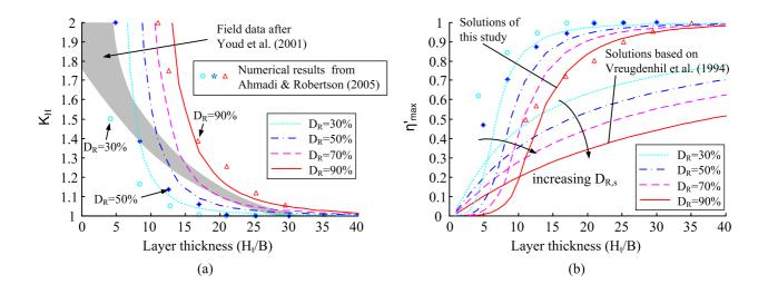
FIG. 18. Comparisons of the parameters for investigation of thin-layer effects: (a)  $K_{H}$ ; (b)  $\eta^{\,\prime}_{max}$
