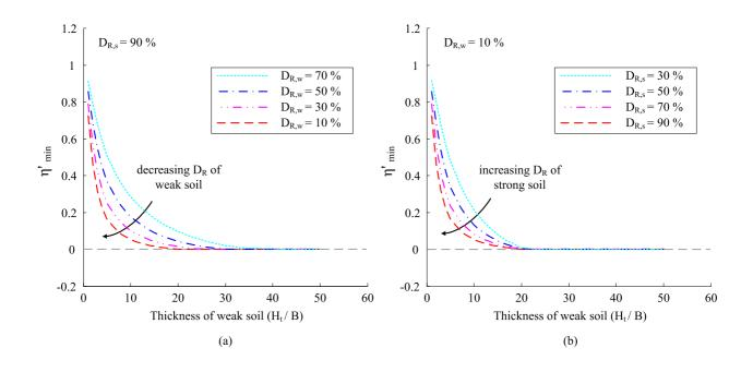
FIG. 17. Variation of the minimum resistance ratio  $\eta'_{min}$  with the thickness of the thin-layer: (a) varying  $D_R$  in weak soil; (b) varying  $D_R$  in strong soil
