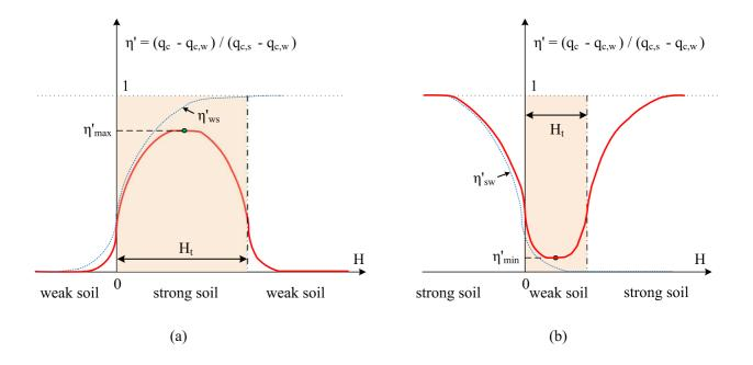
FIG. 11. Schematic of cone tip resistance ratio ( $\eta'$ ) in thin-layered soils: (a) strong soil embedded in weak soils, and (b) weak soil embedded in strong soils
