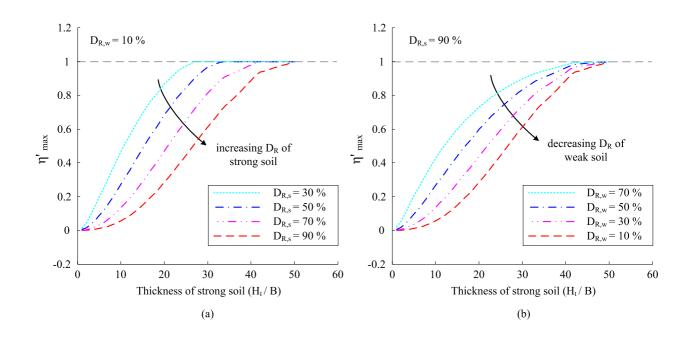
FIG. 14. Strong soil within weak soil: variation of the maximum resistance ratio  $\eta'_{max}$  with the thickness of the thin-layer: (a) varying  $D_R$  in strong soil; (b) varying  $D_R$  in weak soil
