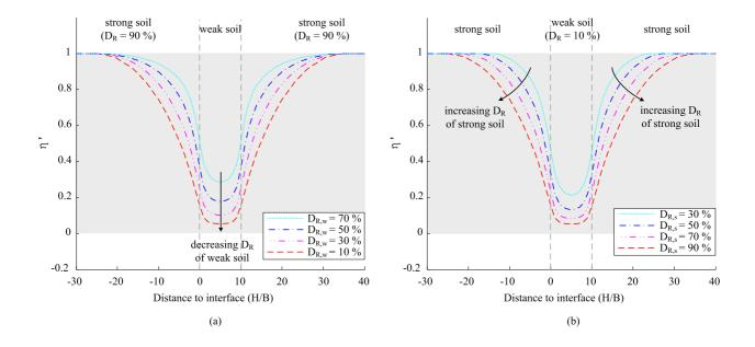
FIG. 16. Resistance ratio curves for thin-layer of weak soil ( $H_t/B = 10$ ): (a) varying  $D_R$  in weak soil; (b) varying  $D_R$  in strong soil
