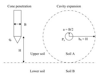
FIG. 4. Schematic of cone penetration and cavity expansion in two-layered soils
