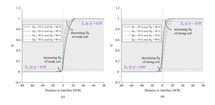
FIG. 7. Cone tip resistance ratio curves in two-layered  $(D_R)$  soils: (a) variation of weaker soil; (b) variation of stronger soil
