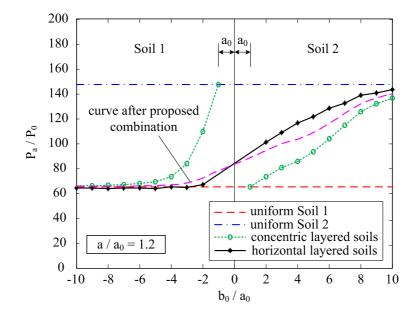
FIG. 3. Cavity pressure with variation of  $b_0\,/\,a_0$  in concentric and horizontal layered model when  $a/a_0=1.2$
