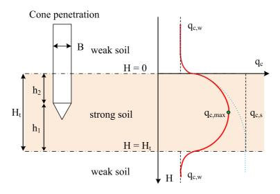
FIG. 10. Schematic of cone penetration in multi-layered soils: strong soil embedded in weak soils
