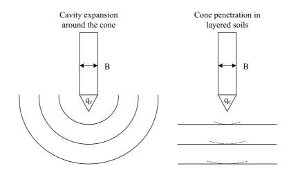
FIG. 1. Comparison of cavity expansion in concentric regions and cone penetration in horizontal layers (adapted from S. M. Sayed and M. A. Hamed, 1987, "Expansion of cavities in layered elastic system." International Journal Journal for Numerical and Analytical Methods in Geomechanics, Vol. 11, No. 1, pp. 203 - 213, ©1999 - 2016 John Wiley & Sons, Inc. Reproduced with permission)
