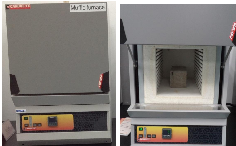
Fig. 2: Carbolite Furnace, shown is the outside and the chamber with a concrete block inside
