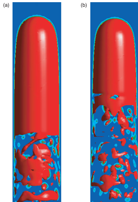
Figure 10. Taylor bubble with (a) 30 kPa over-pressure and (b) 30 kPa under-pressure.
