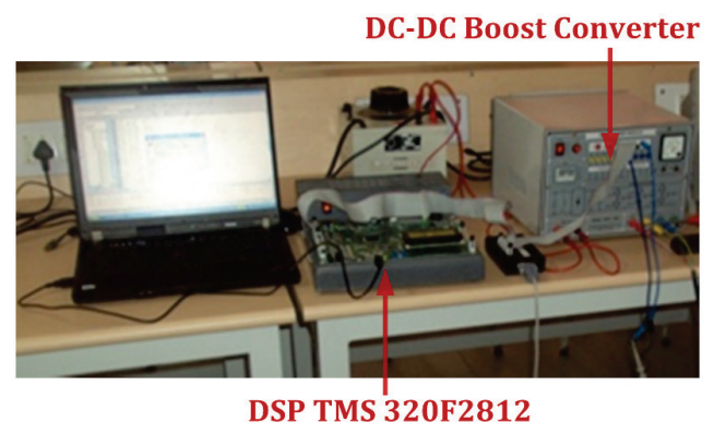
Fig. 8. Hardware prototype module of EHV dc-dc boost power converter with DSP TMS320F2812 processor.
