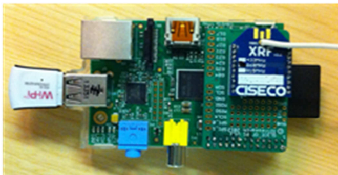
Fig. 2. DTN Pi with 801.11 adapter and XRF receiver for wireless sensors.
