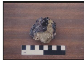
(f) A small fragment of glass furnace floor from Al-Raqqa, Syria with raw purple glass attached (sample RAQ 38). Hundreds of other fragments were found there
