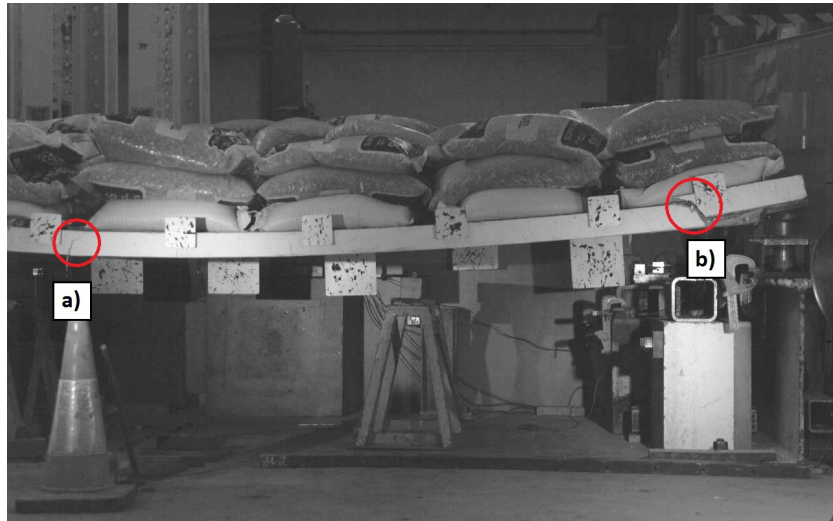
Figure 17: Failure of slab PR-D captured from high speed camera - a) Flexural cracking; b) Shear crack
