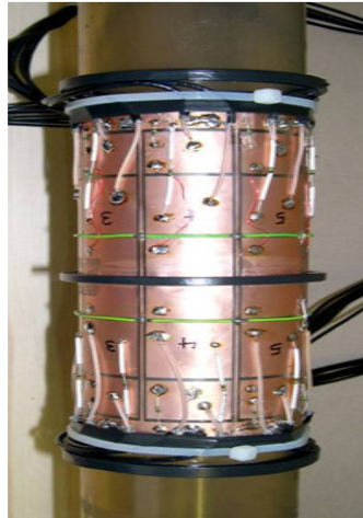
Figure 2: Photo of the Electrical Capacitance Tomography (ECT)
