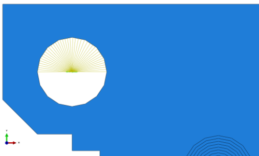
Figure 47. MPC (Multi-Point Constraint) - rigid connection between the centre of the hole and the surrounding nodes of the mesh.
