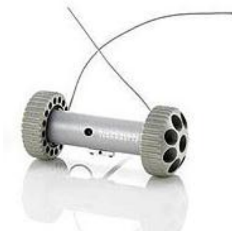
Figure 7 - Recon ThrowBot LE from Recon Robotics ("Recon Scout - Throwbot LE [Image]," 2015)
