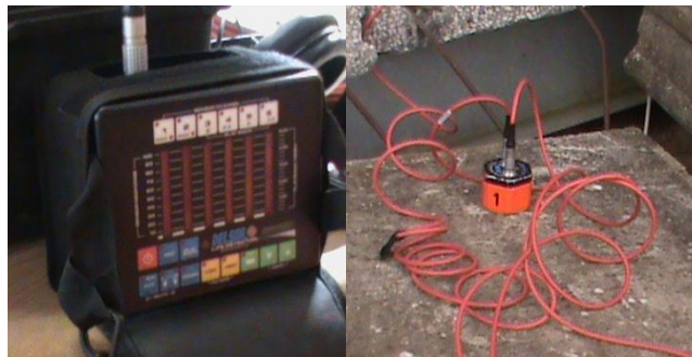
Figure 47 - DELSAR Life Detector LD3 with sensor channel monitor (left) and a sensor on a rubble pile (right)
