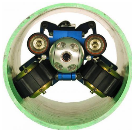
Figure 2 - Pipe crawler Versatrax 150 ("Pipe crawler Versatrax 150 [Image]," 2015)
