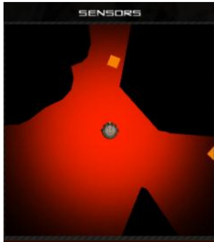
Figure 104 - Top view map from the robot interface with navigation goal points (orange squares)
