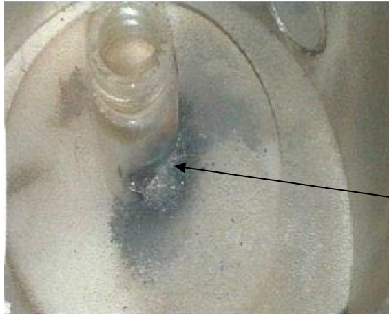
Figure 6-12: Effect of thermal runaway on the reactor in the applicator during microwave pyrolysis of dried polluted soil during preliminary test beyond the timescale used for this experiment.
