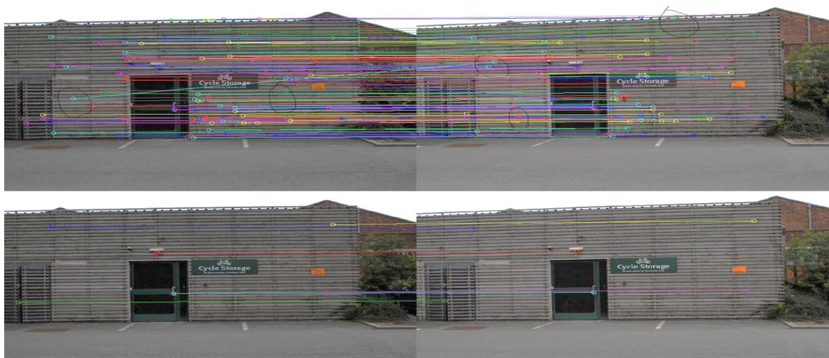
Figure 6. (top) SURF without filtering; (bottom) final common points using the modified SURF
