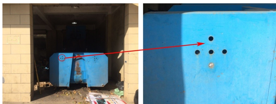
Figure 2. Field photos of a solid waste container in the solid waste transfer station we used for source sampling at Fudan University. Before sampling, an Ogawa passive sampler for \text{NH}_3 is attached on a plastic strip (1.5 m in length). The sampler is fitted into the container through the holes (shown on the right panel).
