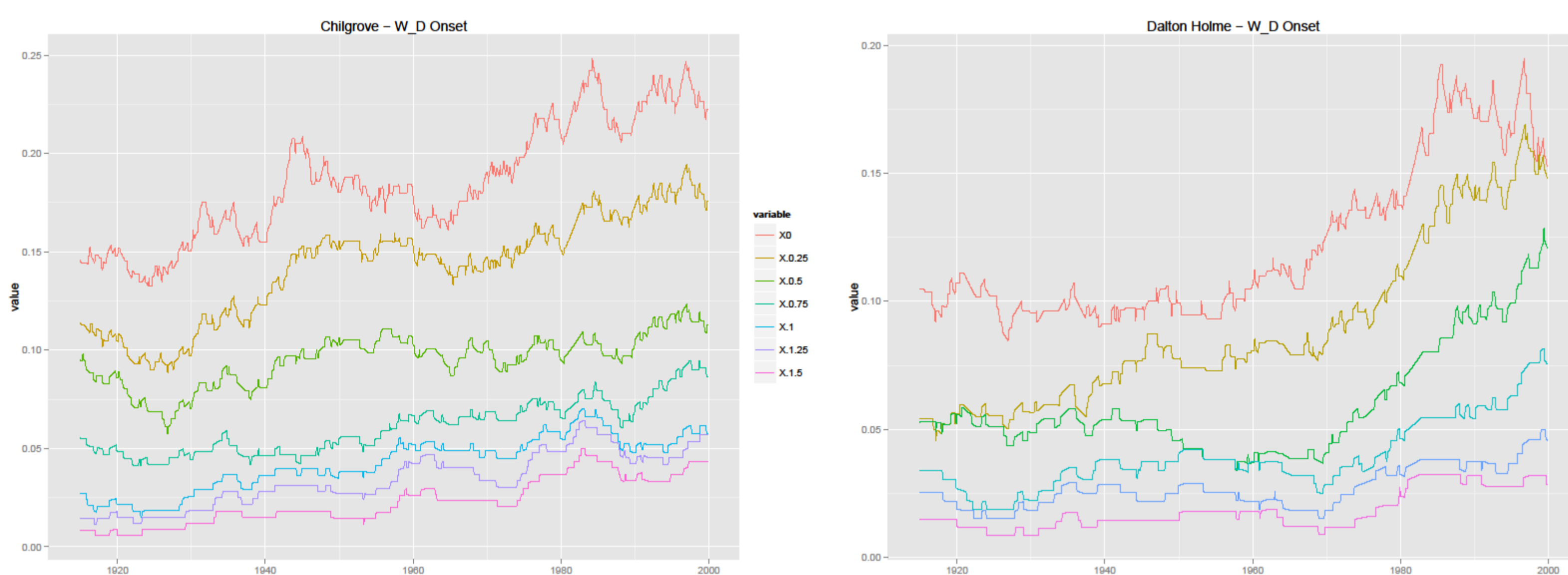
Probability of a 'non-drought : drought' Markov transition, i.e. drought onset, for various SGI thresholds, probabilities derived from a moving 30 year window of observations (data plotted against the centre of the 30 year window).
