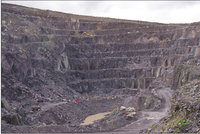
Figure 2. Cambrian slate is currently produced for roofing, architectural and a variety of crushed slate products at Penrhyn Quarry at Bethesda. (Image T Hughes)
