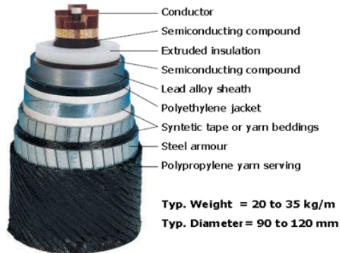
Figure 2.23: Structure of extruded cable [100]
