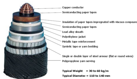
Figure 2.22: The structure of Mass-impregnated (MI) cable [100]
