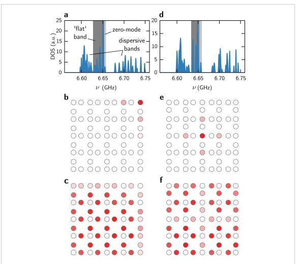
**Figure 2.** Experimental results for the microwave realization of the partial chiral dimerized Lieb lattice, with a defect state localized in the corner ((a)-(c)) or in the center ((d)-(f)). ((a),(d)) Density of states, with the point-defect zero mode shaded in light gray and the flat band shaded in dark grey. ((b),(e)) Spatial distribution of the zero mode. ((c),(f)) Spatial distribution of the flat band.
