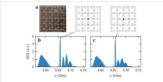
**Figure 4.** (a) Picture of the experimental set-up realizing a dimerized Lieb lattice with identical absorption on the *A* sites, again configured to support a defect state at the center. (b) Density of state of the regular system. (c) Density of state of the disordered system (same configuration as in figure 3). The absorption suppresses the flat-band and extended states, but does not suppress the defect state, which remains localized (insets).
