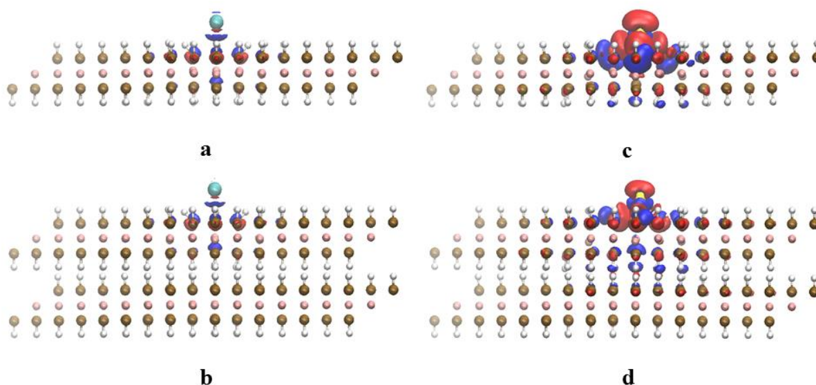
Figure 3: Electron density difference plots of adsorbed \text{Cs}^+ (a, b) and \text{Sr}^{2+} ion (c, d) on 6\times 6_1 (a,c) and on 6\times 6_2 (b,d). The isosurface value was chosen to be 0.0025 a.u. throughout. The red regions are indicative of electron depletion, while the blue regions to electron accumulation. Point charges are not shown. (Mg=pink, O=ochre, H=white, Sr=yellow, Cs=turquoise) 74
