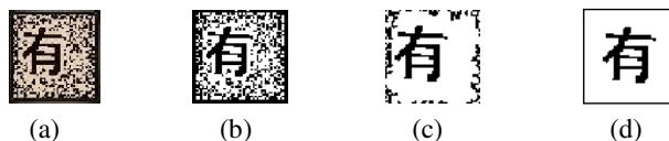
Figure 5: Processing style 1 images. (a) Original; (b) Binarized image; (c) After noise removal; (d) After cropping and rescaling
