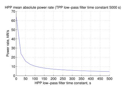
Fig. 6.17 HPP mean absolute power rate with respect to low-pass filter time constant.
