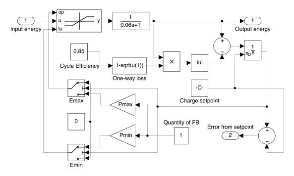
Fig. B.4 The structure of the flow battery model
