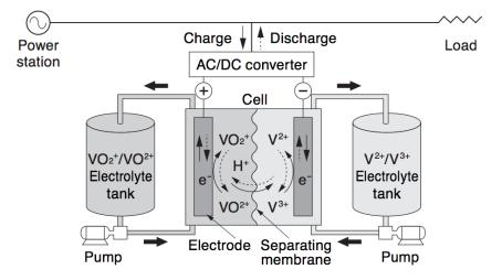
Fig. B.1 Principle and configuration of a flow battery [Shi11]
