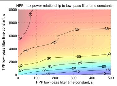
Fig. 6.12 Relationship of required HPP active power reserve with respect to low-pass filter time constants.
