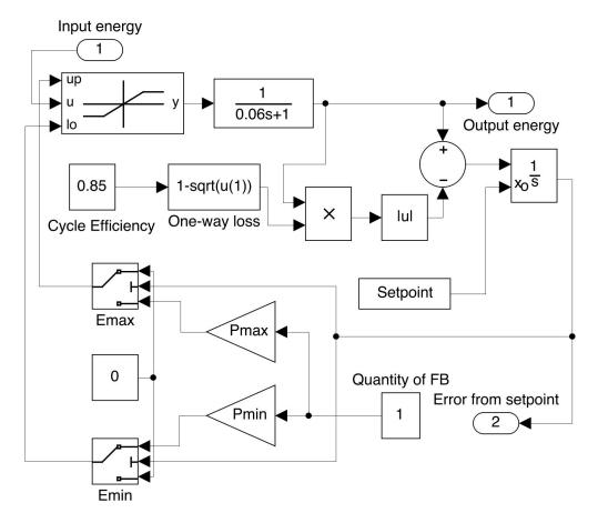
Fig. 6.8 The structure of the flow battery model.
