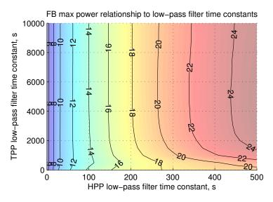
Fig. 6.15 Relationship of required FB active power reserve with respect to low-pass filter time constants.
