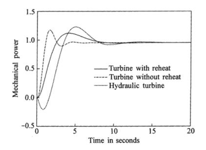
Fig. 6.4 Typical responses of steam and hydraulic units [KBL94].
