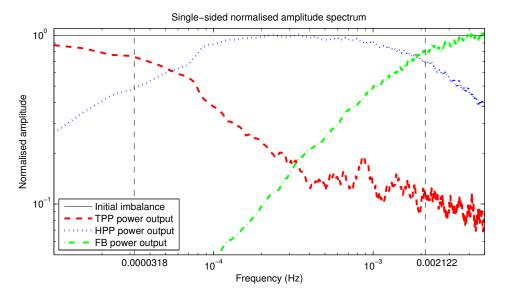
Fig. 6.19 Frequency decomposition of initial wind power and TPP, HPP, FB output powers.
