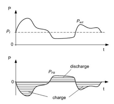
Fig. B.3 The control principle of the FB
