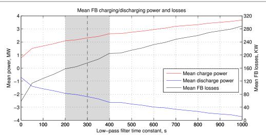
Fig. B.7 Mean FB charging/discharging power and losses
