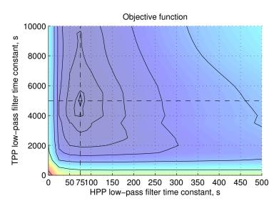
Fig. 6.18 The output of the objective function. A minimum can be seen then time constants are 75 and 5000 for HPP and TPP respectively.
