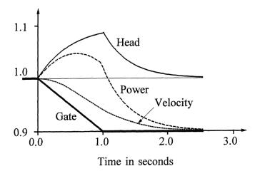
Fig. 6.2 HPP main parameters respect to reduction in gate opening [KBL94].
