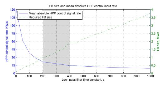
Fig. B.6 FB capacity and mean absolute HPP control input rate
