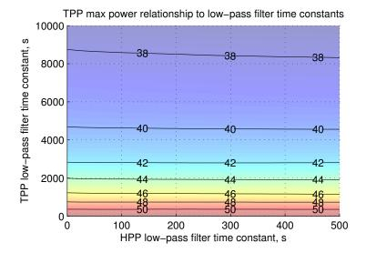
Fig. 6.10 Relationship of required TPP active power reserve with respect to low-pass filter time constants.
