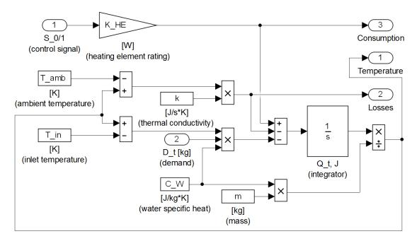
Fig. 5.2 Thermal water heater block diagram model.
