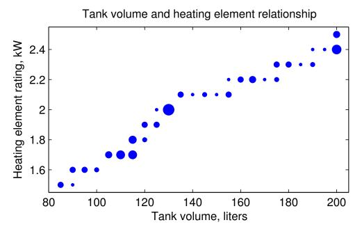
Fig. 5.5 Water heater tank size and heating element power rating relationship.
