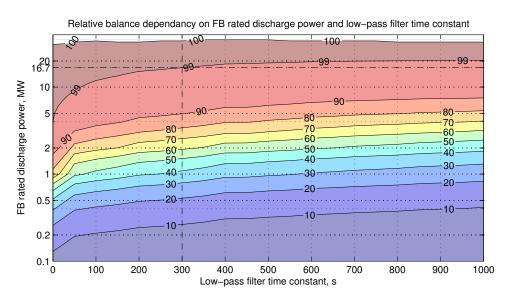
Fig. B.11 Relative balance dependancy on FB rated discharge and LPF time constant.
