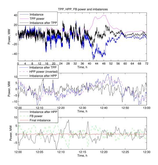
Fig. 6.20 Balancing the difference between actual and forecasted wind power with thermal power plant, hydro power plant and flow battery.
