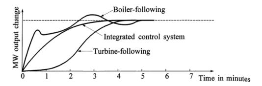
Fig. 6.3 TPP power output in respect to control mode [KBL94].
