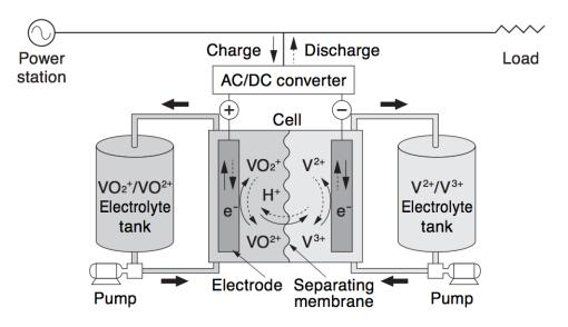
Fig. 6.5 Principle and configuration of a flow battery [Shi11].
