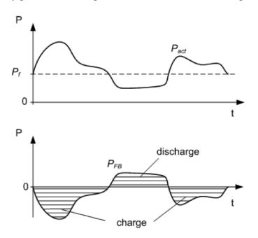
Fig. 6.7 The control principle of the FB.  $P_{act}$  - actual wind power,  $P_f$  - forecasted wind power,  $P_{FB}$  - power of flow battery.
