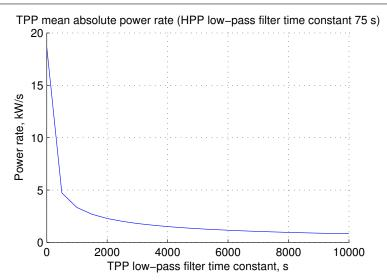
Fig. 6.16 TPP mean absolute power rate with respect to low-pass filter time constant.
