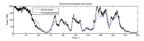
Fig. 6.9 The forecasted and actual wind power for a installed capacity of 222 MW from 1st to 10th of February, 2014.
