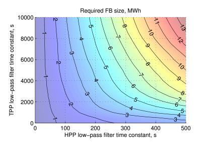
Fig. 6.14 Relationship of required flow battery capacity with respect to low-pass filter time constants.
