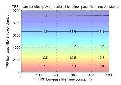
Fig. 6.11 TPP mean absolute power relationship with respect to low-pass filter time constants.
