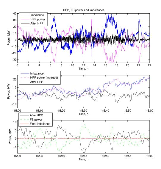
Fig. B.8 Balancing the difference between actual and forecasted wind power with hydro power plant
