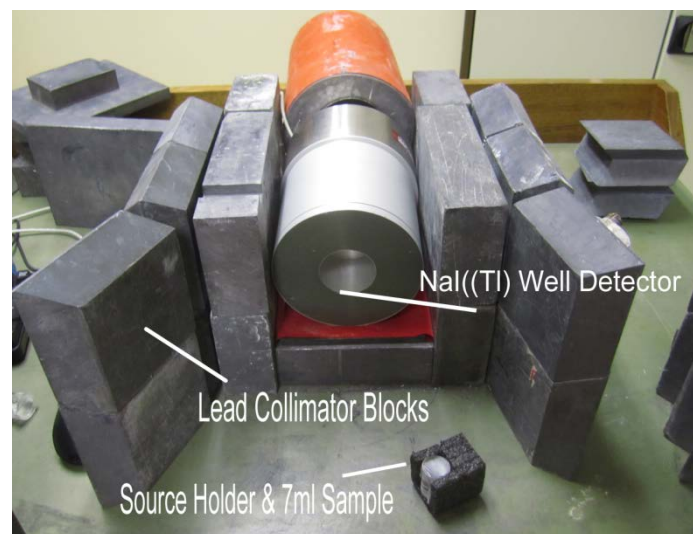
Figure 2. The NaI(Tl) well counter used in this work. The lead blocks have been removed from the top of the instrument to provide a better view of the detector.
