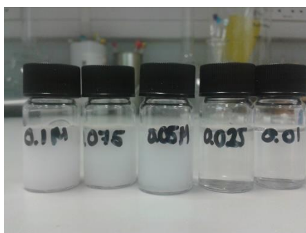
Figure 3.7 Solutions of 1% SL with different concentrations of NaCl and 0.01 M NaOAc. The concentrations of salt were 0.1 M (gel), 0.075 M (gel), 0.05 M (gel), 0.025 M (slight gel at top of vial) and 0.01 M (solution). All samples had been left overnight before a photo was taken.
