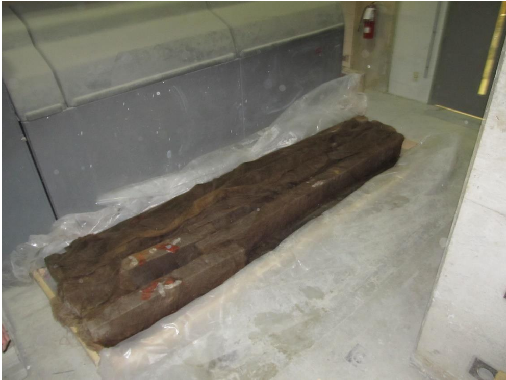
Fig. 3 Specimens covered with wet burlap
