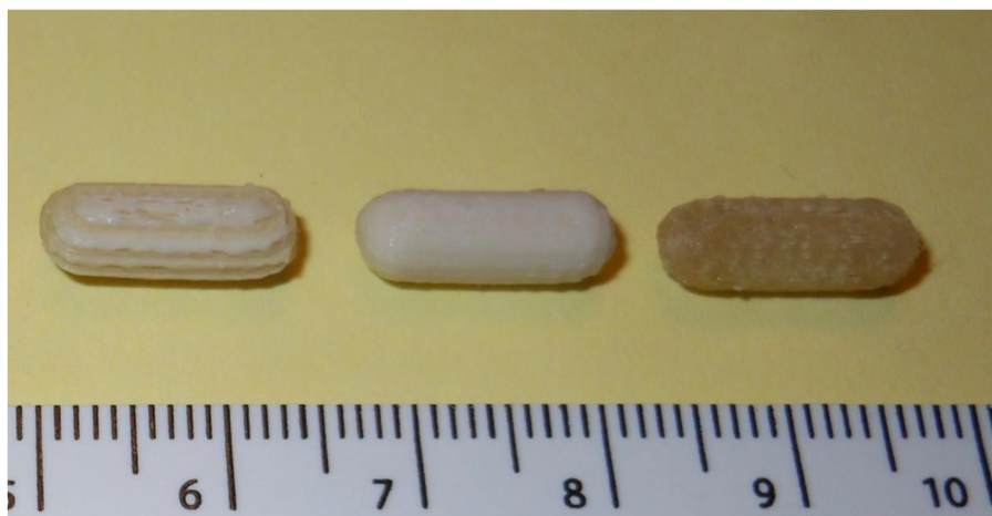
Figure 4. Images of the 3D printed caplets: from left to right, multilayer device of 8.2% paracetamol-PVA 9.5% caffeine-PVA, DuoCaplet of 9.5% caffeine-PVA (outer) 8.2% paracetamol-PVA (core) and DuoCaplet of 8.2% paracetamol-PVA (outer) 9.5% caffeine-PVA (core)
