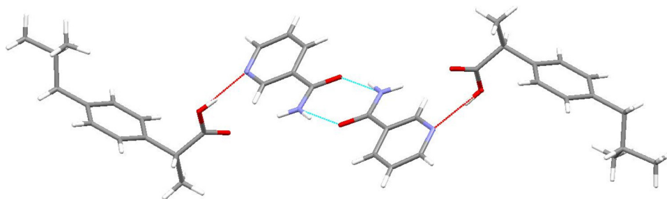
Fig. 1. 1:1 IBU-NIC co-crystal molecular structure. Hydrogen bonding is shown by light blue and red dashed lines. (For interpretation of the references to colour in this figure legend, the reader is referred to the web version of this article.)
