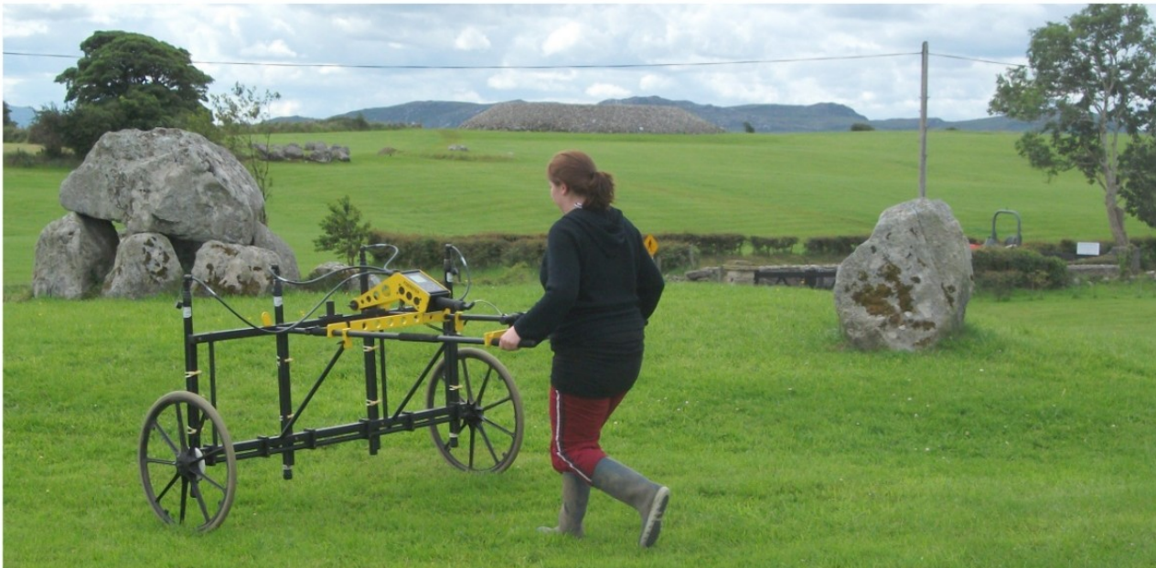
Figure 21. Cart mounted magnetometer arrays.
