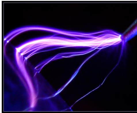
Figure 2.30 Electrical discharge during corona discharge ( www.dynetechology.co.uk ).
