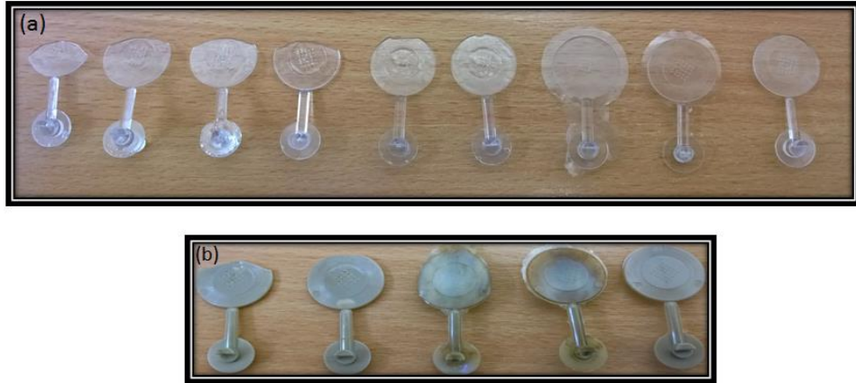
Figure 3.29 Parts produced during short shot optimisation (a) Lexan (b) PEEK.
