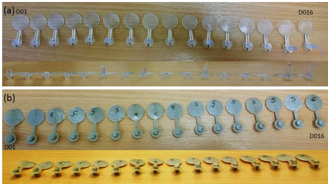
Figure 3.33 Photograph of the parts produced with different design order showing the variation in the melt cushion. (a) Lexan (b) PEEK.
