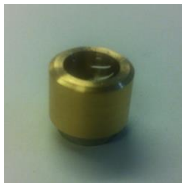
Figure 3.17 Photograph of the holder with the MN insert used for PDMS replication.
