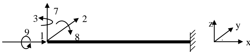
Fig. 3 A cantilever model for calculating the relations between the nodal actions and basic deformation parameters.
