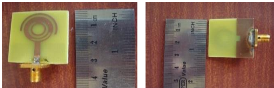
Fig. 10 Fabricated antenna (a) front view and (b) rear view
