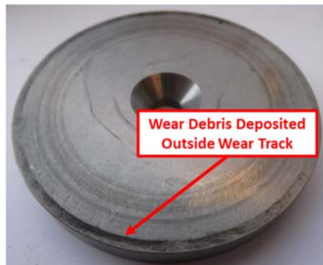
Figure 16: Steel Disc after a Test but before Cleaning (PEK at 8ms -1 and 1MPa) showing Wear Debris removed from the Contact Area
