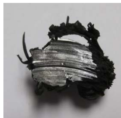
Figure 9: PEEK Pin after Failure During Phase 2 at 1MPa
