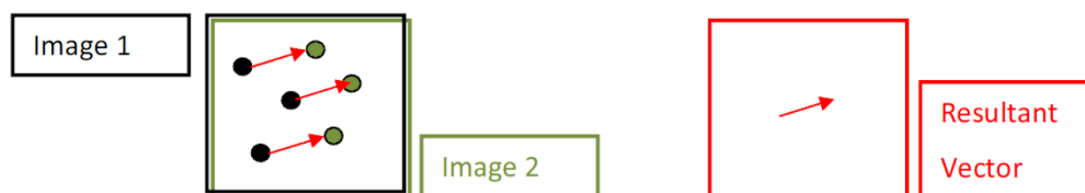
Figure 4-8: Cross-correlation of particle images to obtain velocity vector (Nichols, 2008)
