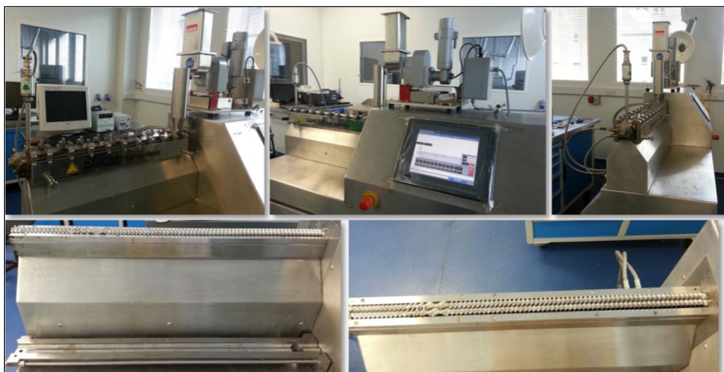
Figure 3.2 Different views of Pharmalab co-rotating 16 mm twin screw extruder
