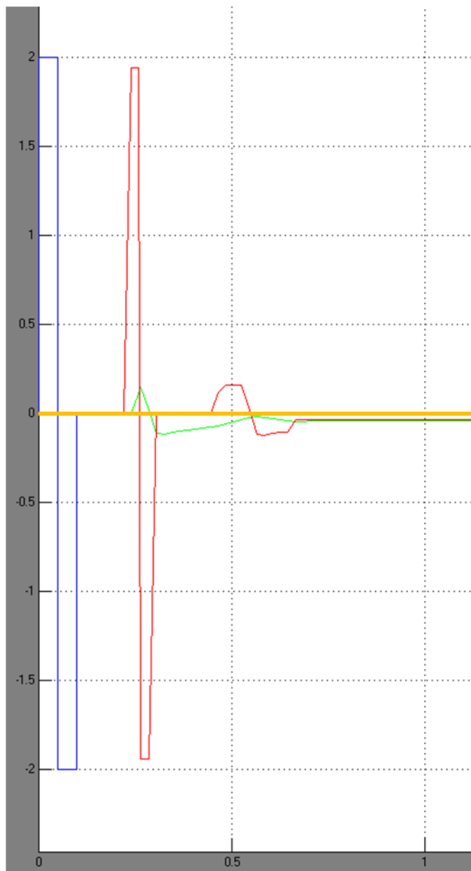
Figure 6-11: The double AR (green trace) predicted by Khosroyani and Hung (2002), in response to the 50 ms, 2 D stimulus of this experiment (dark blue square wave). The red trace is the accommodation signal generated by the “open-loop” component of the model. It follows the AS after a latency interval and is finally attenuated by the biomechanical response. The orange trace (at zero) is the signal generated by the “closed-loop” component of the model. In the case of such large and rapid changes, this component is not affected. (It does contribute to the simulated response to other stimuli from this experiment.)
