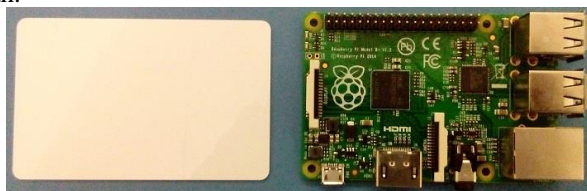
Gambar 1. Credit card sized computer (CCSC).
