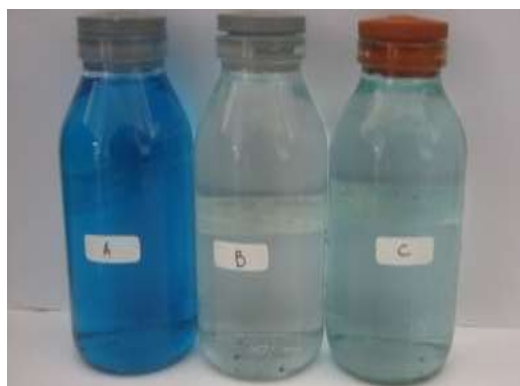
Figure 3. Photoactivity of ZnO thin film for 10 ppm dye MB solution: (A) Without treatment, (B) with treatment using ZnO thin film and stirring of 3 hour, and (C) with treatment using ZnO thin film and without stirring.
