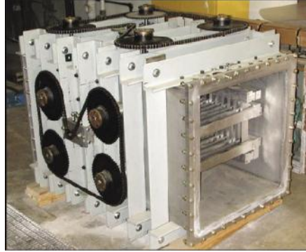
Figure 1.4: Internal view of microwave dryer [10]
