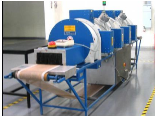
Figure 5.2: Continuous microwave belt furnace [13]
