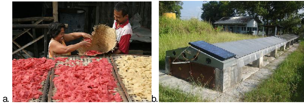
Figure 1.2: Direct sun dryer (a) and solar tunnel dryer (b) developed in Indonesia [7]
