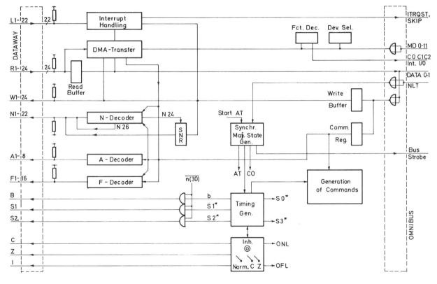
Fig. 1 Block Diagram of Single-Crate Controller for PDP-8/E (SCC-8/E)\*
