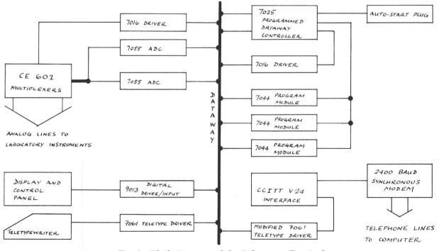
Fig. 1 Block Diagram of the Laboratory Terminal
