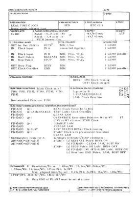
Fig. 1 Form for Describing the Characteristics of CAMAC Equipment
