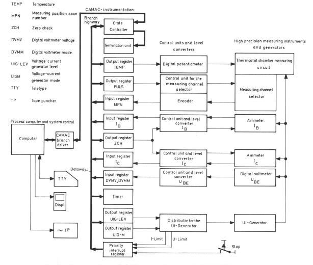
Fig. 1 Computer Controlled Measuring System with CAMAC-Instrumentation
