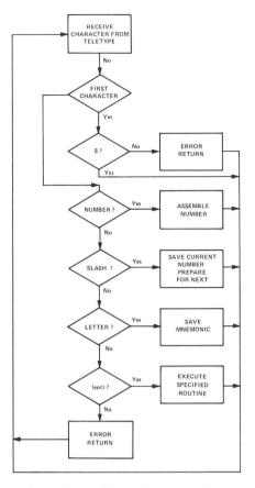
Fig. 1 Flow Chart of Basic Monitor
