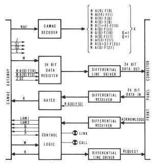
Fig. 2 Transmitter-Receiver Module Block Diagram
