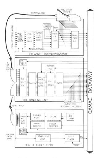
Fig. 1 Block Diagram and Interconnection of the Described CAMAC Modules (Time-of-Flight Mode)
