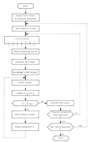
Fig. 2 Flow Diagram for the Measurement of Transistor Characteristics
