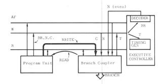
Fig. 2 Data Flow Paths — Branch Mode Operation
