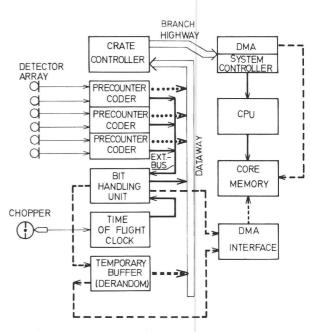
Time-of-Flight Configuration with Several Fig. 2 Possible Paths of Data Transfer into Core Memory
