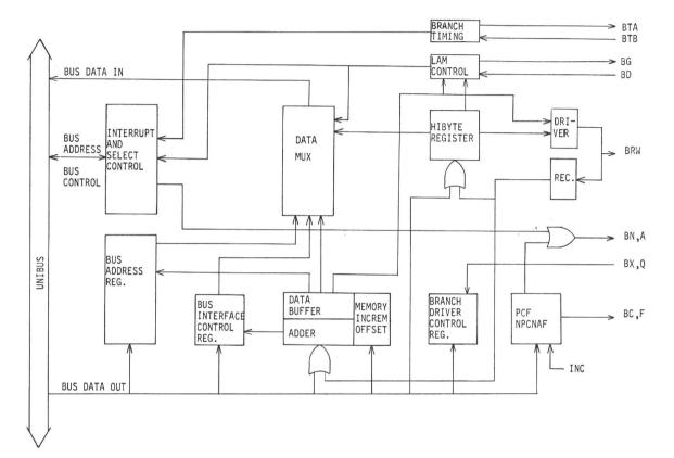
Fig. 1 Block Diagram of the CA11-C CAMAC Interface
