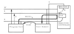
Fig.1 Data Flow Paths — CAMAC Mode Operation
