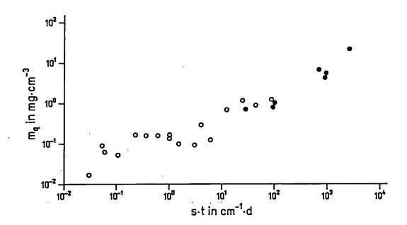
Figure 1. Amount of reacted glass per leachant volume m as a function of the product sot for the corrosion of the HLW<sup>q</sup>glass SON 68 in solution 1 at 190 °C; s: ratio of glass surface area to leachant volume; t: corrosion time;
