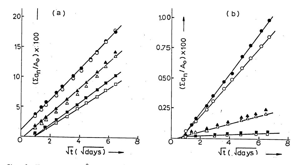
Figure 3. Elution curves at 30°C of (a) NaCl or (b) SrSO<sub>4</sub> from duplicate specimens (∿7 mm thick) of salt-loaded epoxy resin. Salt content (% vol): 12 (□, ■), 25 (Δ, ▲), 40 (o, ●).
