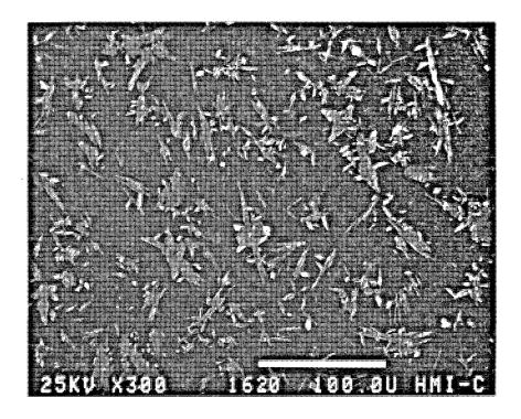
Figure 1 SEM micrograph of HLW glass SM513LW11 annealed at  $620^{\circ}$ C for 100 days. (White bar = 100  $\mu$ m)
