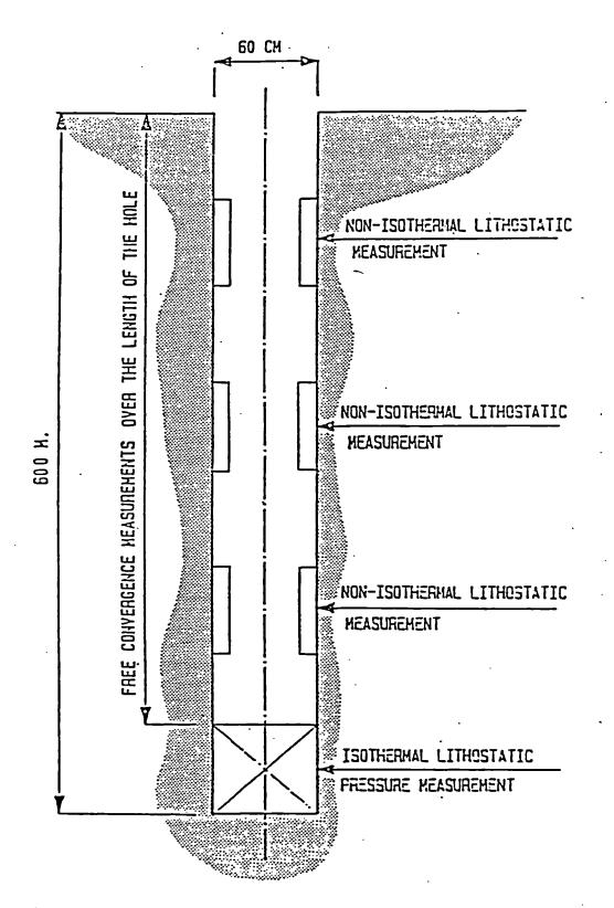
Fig. 1 : Sketch of the 600 m bore hole measurement set up.
