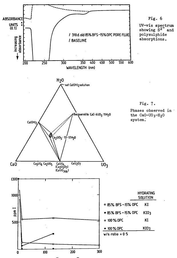
Fig. 8. Sorption of I and IO3 in cement and slag-cement pastes.
