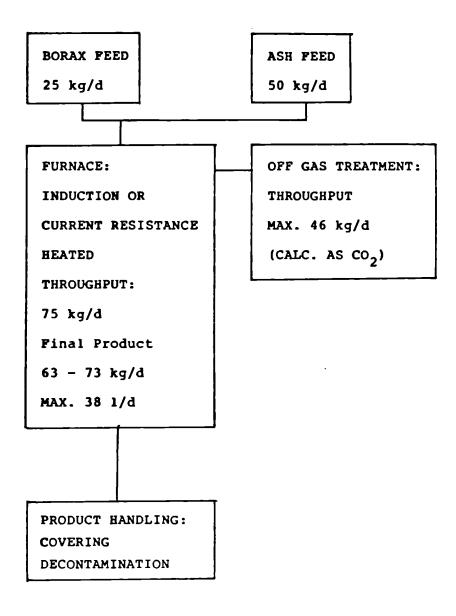
Fig. 1: Flow diagram of a melting process (1000 °C, 50 % Borax)
