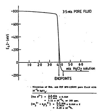
Fig. 5. Typical titration curve for aqueous sulphide determination.
