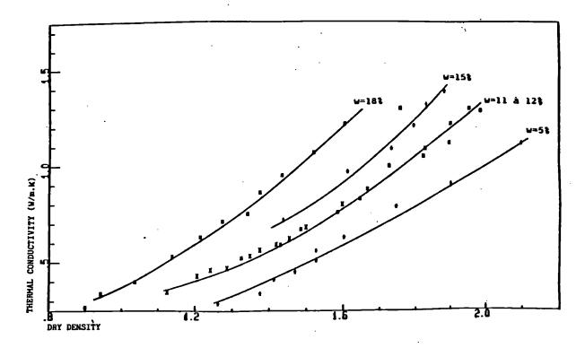
Figure 1 : Thermal conductivity as a function of dry density for reference 4a (20°C) (w = Water content)
