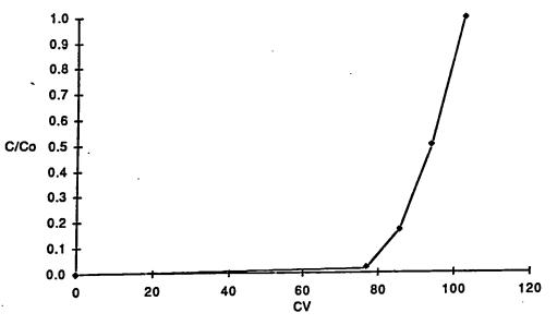
Fig.3 IE-96 Zeolite break-through curve
