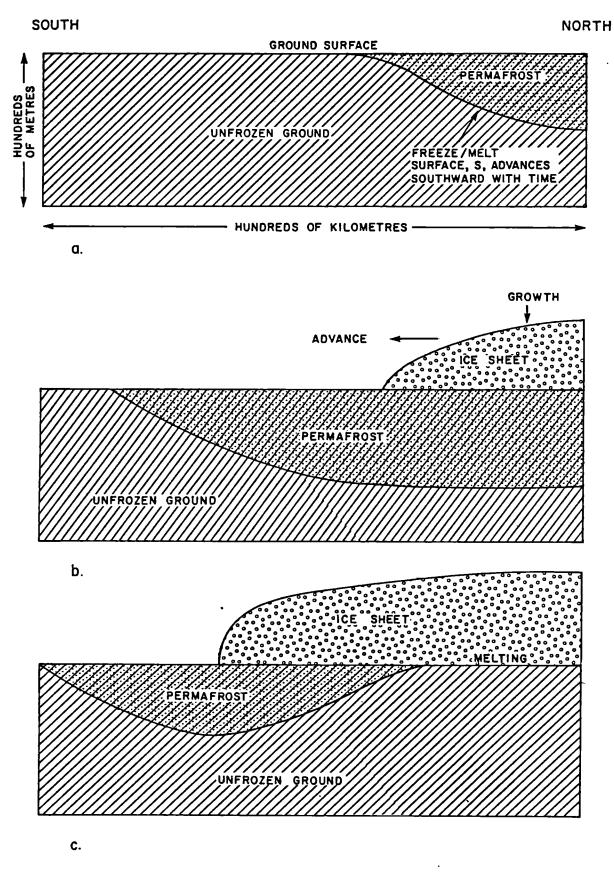
FIGURE I SCHEMATIC ILLUSTRATION OF PERMAFROST DEVELOPMENT.
