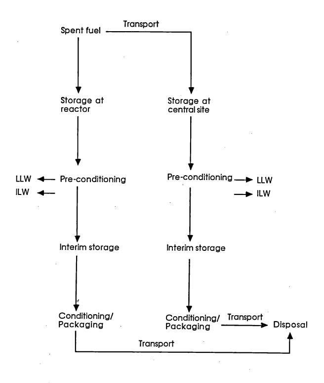
Figure 1 Schematic diagram of direct disposal options
