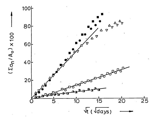
Figure 1. Elution curves of Cs from duplicate cemented specimens containing inactive Cs<sub>2</sub>SO<sub>4</sub> (3.4% wt) at 70° (Series B; •, •) or 30°C (Series A,C; o, σ, ∇, Δ) or Cs-137 (10 µCi/sample), CsNO<sub>3</sub> (0.017% wt) and NaNO<sub>3</sub> (8% wt) at 30°C (Series D; o, •). Sample thicknesses: 1.2 cm (Series C; ∇,Δ) or 4.0 cm (Series A,B,D; o, σ, •, •, •, •, •).
