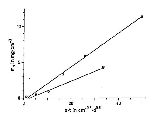
Figure 2. Amount of reacted glass per leachant volume,  $m_B$  (determined by boron analysis of leachate) as a function of  $\sqrt{s \cdot t}$  for the corrosion of the HLW glass SON 68 in solution 3 at 150 °C; □: 30 d; 0 : 120 d
