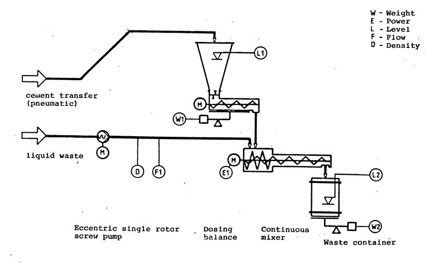
Fig. 3: Flowsheet continuous mixer Process instrumentation Conditioning of ashes from combustion plants in special melting furnaces
