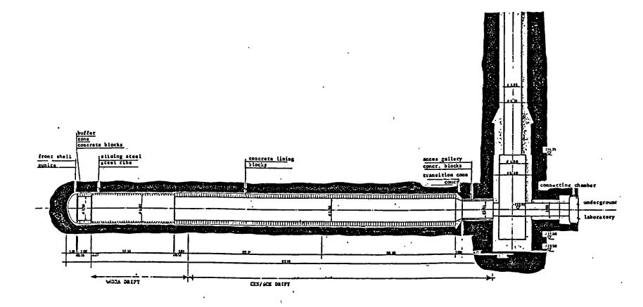
Fig. 1. Scheme of the test drift (as built)
