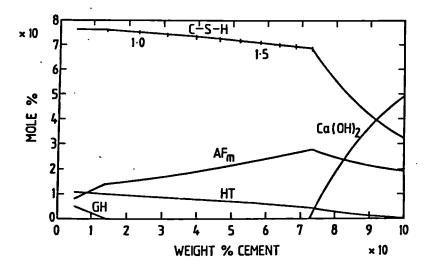
Fig. 2. Phase distribution in slag-cements
