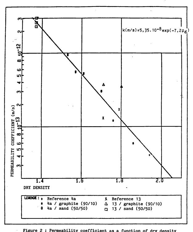
Figure 2 : Permeability coefficient as a function of dry density
