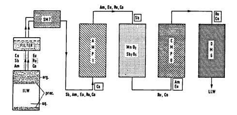
Fig. 1: Flowsheet of the chromatographic decontamination of ILW solutions.
