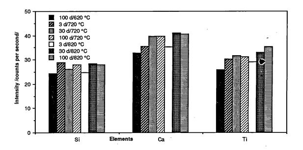
Figure 2a X-ray intensities of elements from SEM-EDS analysis of the annealed HLW glass SM513LW11. Annealing times: 3, 30 and 100 days. Annealing temperatures: 620, 720 and 820°C. From analysis of the small, bright crystals in Figure 1.
