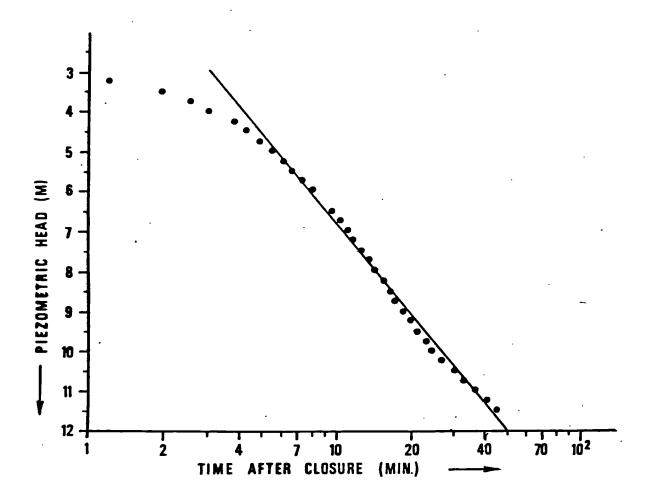
Figure I. Results of a recovery test on an artesian well.
