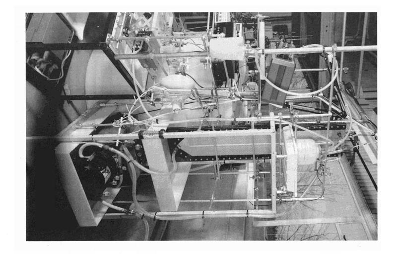
Figure 2 0.1 m<sup>3</sup>/h EIX treatment cell.
