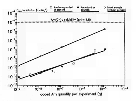
Fig. 1: Am-241 equilibrium concentrations in the system cemented waste form/Q-brine at room temperature for samples with different Amcontent (2 g cement, 30 ml Q-brine).
