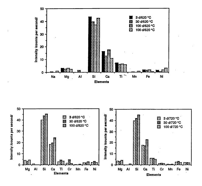
Figure 2b X-ray intensities of elements from SEM-EDS analysis of the annealed HLW glass SM513LW11. Annealing times: 3, 30 and 100 days. Annealing temperatures: 620, 720 and 820°C. From analysis of the large, dark crystals in Figure 1.
