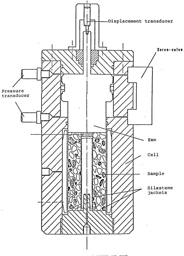
Fig. 2 : SC HEMATIC VIEW OF THE "THICK TUBE" CELL
