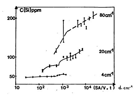
FIGURE 1 : SILICON CONCENTRATION VERSUS (SA/V.t) FOR DIFFERENT SA/V RATIOS (2nd TEST SERIES)
