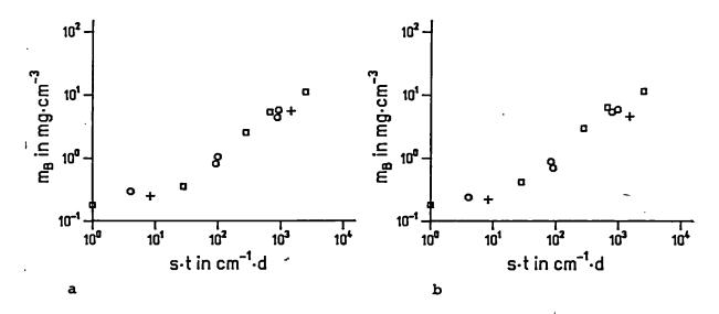
Figure 3. Amount of reacted glass per leachant volume,  $m_B$  (determined by boron analysis of leachate) as a function of solution of the corrosion of the HLW glass SON 68 in solution 1 (a) and solution 2 (b) at 190 °C; \_: 30 d; 0 : 120 d;
