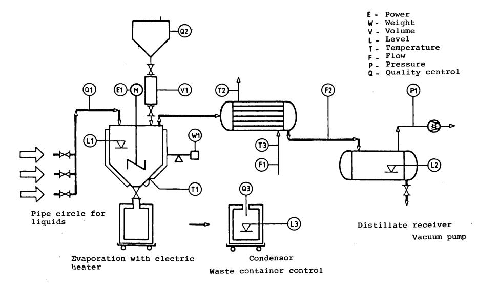
Fig. 1: Flowsheet ROBE product relevant process instrumentation
