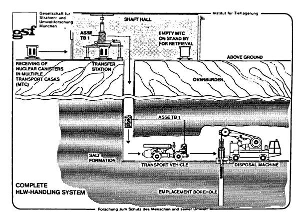
Fig. 2: HAW Handling System
