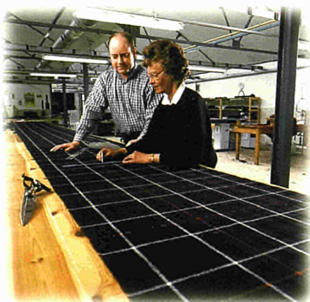
‘Marking out’ the 8 metres of cloth needed to make an adult man’s kilt
