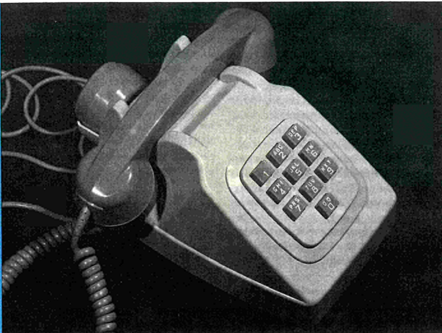
Figure 2: Push-button telephone set. The use of a keyboard instead of a dial has the following advantages: —easier, quicker handling, —at the exchange, reduction in the number of parts that are used only during "dialling", —lower rate of "dialling" errors, —possibility, once the connection is made, of using the keys to communicate with a computer, for instance.
