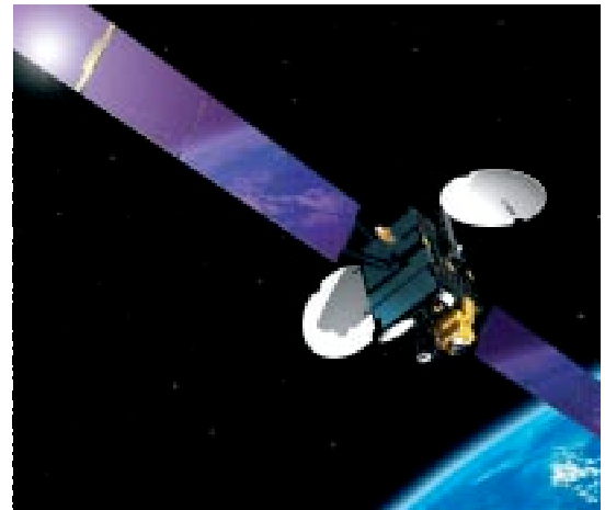
Launched in July 2001, the Artemis (Advanced Relay and Technology Mission Satellite) communication satellite is an intercommunication relay station operating between terrestrial emitting stations and mobile posts. Its new laser transmitting technology also enables it to test inter-satellite communications. © ESA
