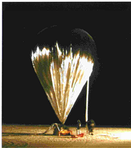
Inflating the helium or hydrogen balloons at Esrange prior to launching them on a journey through the stratosphere of several hundred kilometres at altitudes of over 30 000 metres.
