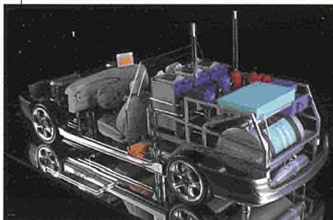
Fuel cell developed by the FEVER project. The only waste emitted by this 100% clean system of energy production: water.
