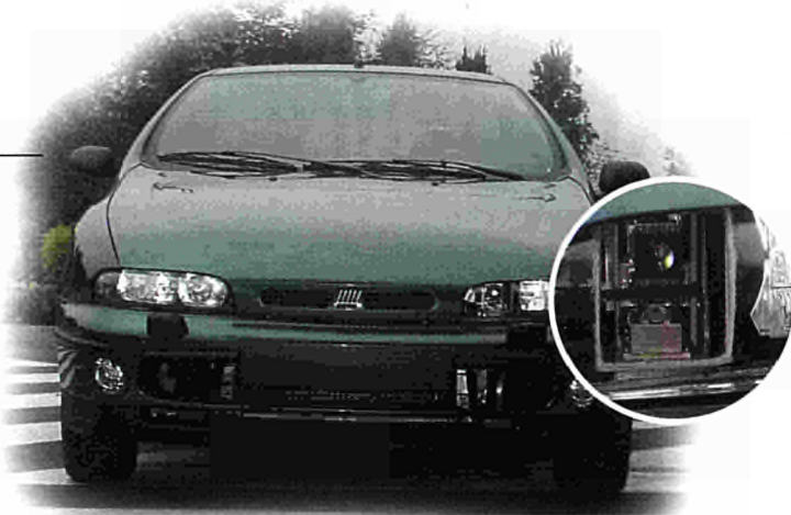
CSEM's laser scanning range sensor is accurate, robust and compact. A prototype (below) was built into the left headlamp of a Fiat Brava (left and inset). CSEM; Centro Ricerche Fiat SpA
