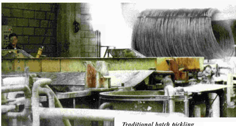
Traditional batch pickling of a two tonne coil of steel wire rod
