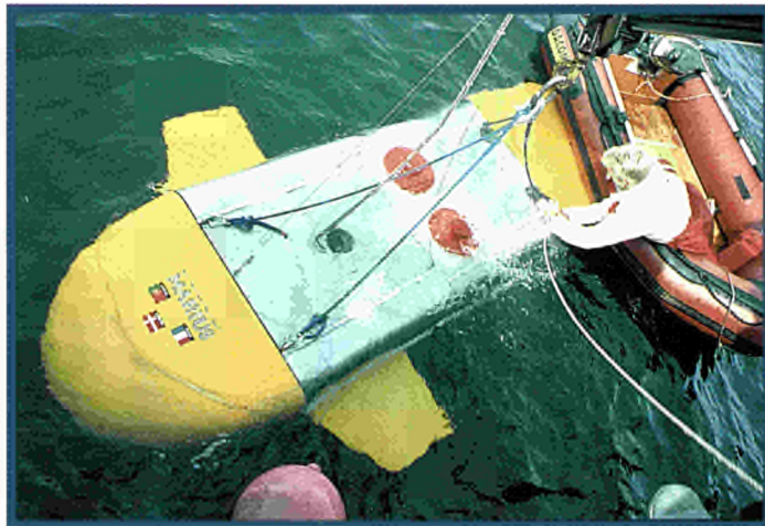
The MARIUS unmanned underwater vehicle undergoing sea trials in 1993.
